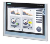
SIMATIC HMI TP1500 Comfort, Comfort Panel, touch operation, 15" widescreen TFT display, 16 million colors, PROFINET interface, MPI/PROFIBUS DP interface, 24 MB configuration memory, WEC 2013, configurable as of WinCC Comfort V14 SP1 with HSP, ambient temperature up to 50 °C (up to 55 °C with restrictions)
