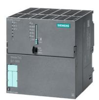
SIMATIC S7-300 CPU 319-3 PN/DP, Central processing unit with 2 MB work memory, 1st interface MPI/DP 12 Mbit/s, 2nd interface DP master/slave 3rd interface Ethernet PROFINET, with 2-port switch, Micro Memory Card required
