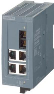
SCALANCE XB004-1 unmanaged Industrial Ethernet Switch for 10/100 Mbit/s; for setting up small star and line topologies; LED diagnostics, IP20, 24 V AC/DC power supply, with 4x 10/100 Mbit/s twisted pair ports with RJ45 sockets; 1 x 100 Mbit/s multimode glass fiber-optical cable port with SC socket; manual available as a download .
