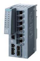
SCALANCE XC206-2SFP manageable Layer 2 IE switch; IEC 62443-4-2 certified; 6x 10/100 MBit/s RJ45 ports; 2x 100/1000 Mbit/s SFP; 1x console port; diagnostics LED; redundant power supply; temperature range -40 °C to +70 °C; assembly: DIN rail/S7 mounting rail/wall Office redundancy functions features (RSTP, VLAN,...); PROFINET IO device; Ethernet/IP-compliant; C-plug slot;
