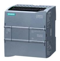
SIMATIC S7-1200, CPU 1211C, compact CPU, DC/DC, onboard I/O: 6 DI 24 V DC; 4 DO 24 V DC; 2 AI 0-10 V DC, power supply: DC 20.4-28.8 V DC, program/data memory 75 KB
