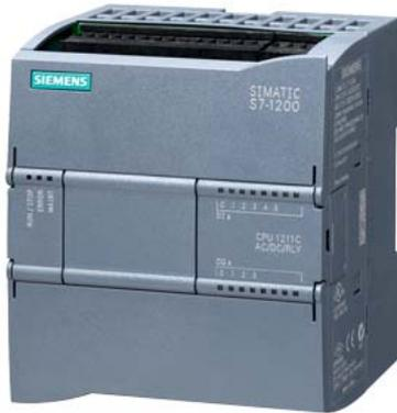
SIMATIC S7-1200, CPU 1211C, compact CPU, AC/DC/relay, onboard I/O: 6 DI 24 V DC; 4 DO relay 2 A; 2 AI 0-10 V DC, power supply: AC 85-264 V AC at 47-63 Hz, program/data memory 75 KB
