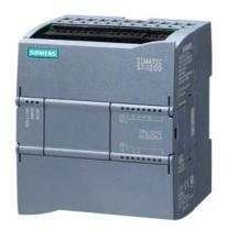
SIMATIC S7-1200, CPU 1211C, compact CPU, DC/DC/relay, onboard I/O: 6 DI 24 V DC; 4 DO relay 2 A; 2 AI 0-10 V DC, power supply: DC 20.4-28.8 V DC, program/data memory 75 KB
